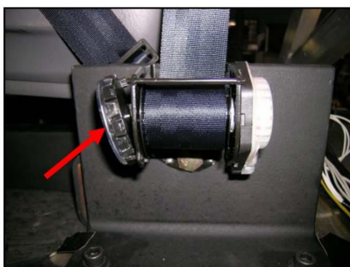
Photograph 21 - S080327 Post-test Partial separation of spring cover on seatbelt retractor
