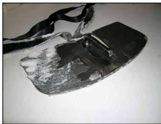
Photograph 12 Metal plate inside cushion
