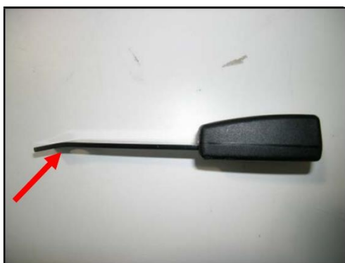
Photograph 23 - S080327 Post-test Deformation rigid buckle on seatbelt assembly
