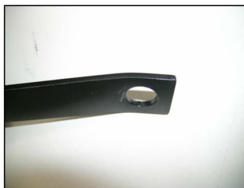
Photograph 24 - S080327 Post-test Detail of rigid buckle
