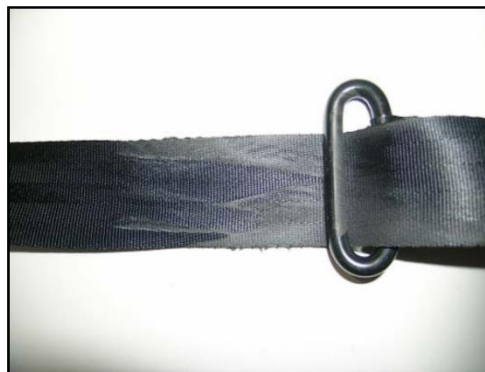
Photograph 20 - S080327 Post-test Abrasion of seatbelt webbing through sash guide
